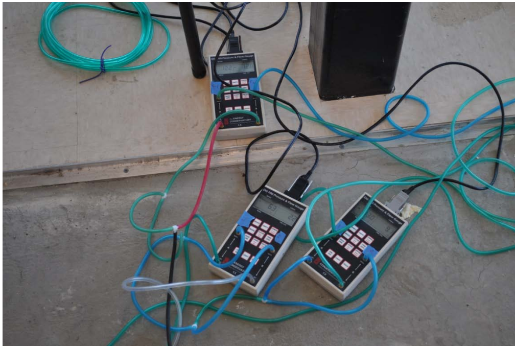
Figure 2. DG700 micromanometers. The colored tubing runs to the exterior locations. The short pieces of tubing tee'd together lead to an indoor location away from the fan location. This is to prevent air movement near the fans from interfering with measurement accuracy.
