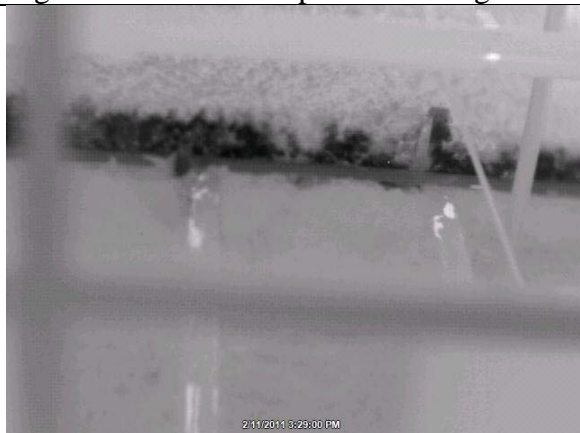
Figure 13 Another location of the showing the air leak at the top of the wall demising wall between garage and conditioned space. The bright vertical lines are infrared reflecting off the shiny steel studs.
